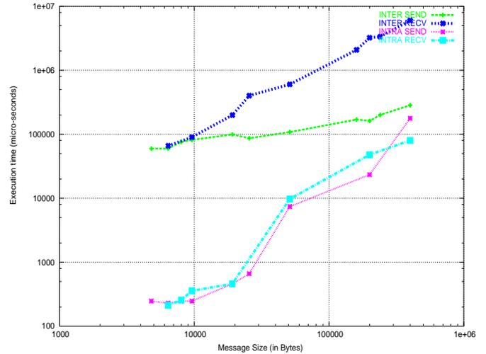
**Figure 4.** Inter and Intra cluster Communication Times for Different Message Sizes
